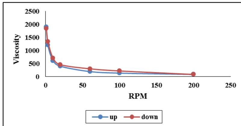
**Fig (8) Rheological properties of (4%) CMC Thickener**
