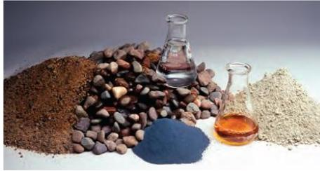
Figure 1 Concrete components.
