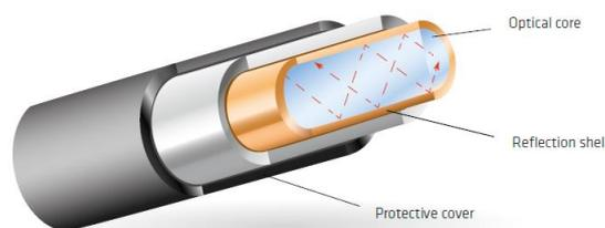
Figure 3 shows the different parts of optical fibers
