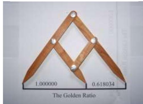
Figure 2: golden ratio mean gauge
